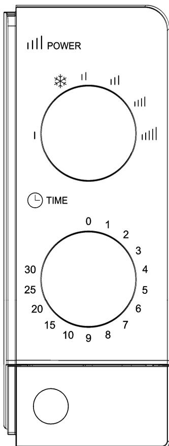
The control panel consists of two function operators. One is a timer knob, and another a power knob.
